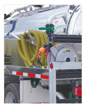
Our portable restroom trucks come standard with retractable hose reel, work lights, hard piped primary line and tiger tail setup.
